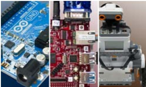
*Simulink built-in support for prototyping, testing, and running models on low-cost target hardware, including Arduino®, LEGO®MINDSTORMS® NXT, and BeagleBoard.*
